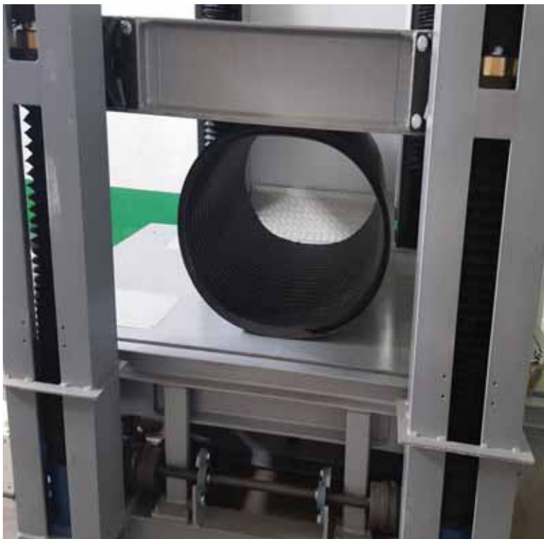
Ring Stiffness Testing of Plasco Weholite Pipes according to ISO 9969 Standard
