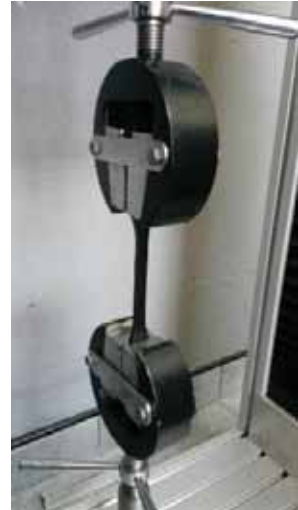
Advanced raw material property testing equipment at Plasco used for testing HDPE materials (from left) : Oxidation Induction Time tester, Tensile properties tester.
