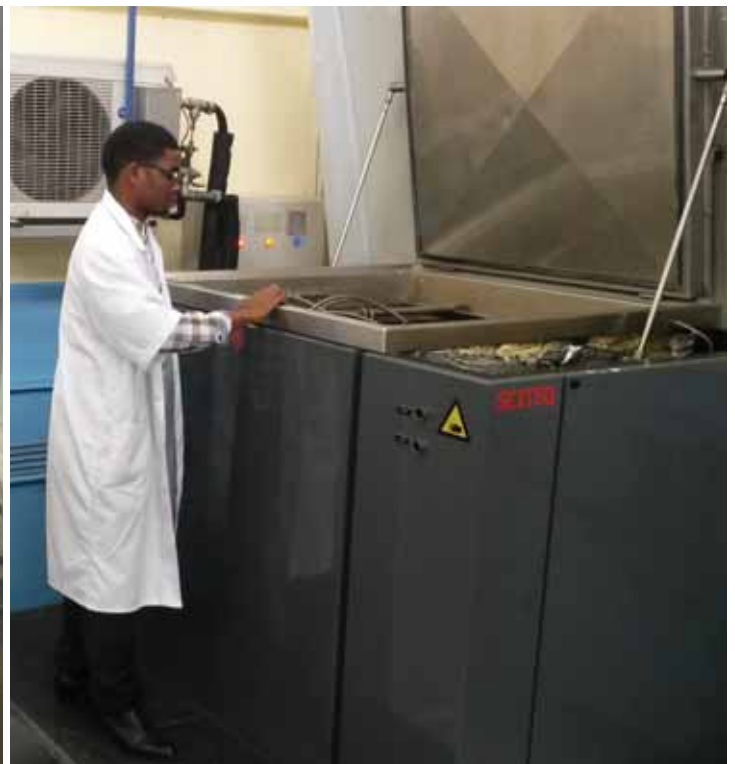
Automatic Hydrostatic pressure test equipment and Thermo-Controlled tanks to execute precise pressure tests at 20°C or 80°C as per international standards.
