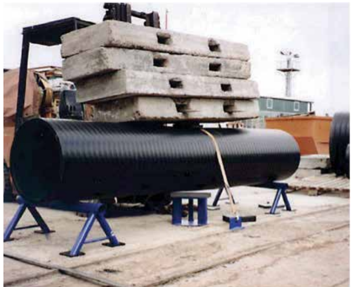
Lengthwise stiffness test for a DN/ID 600mm, SN4 pipe. Load 29kN, deflection 30mm, pipe deformation 54mm.
