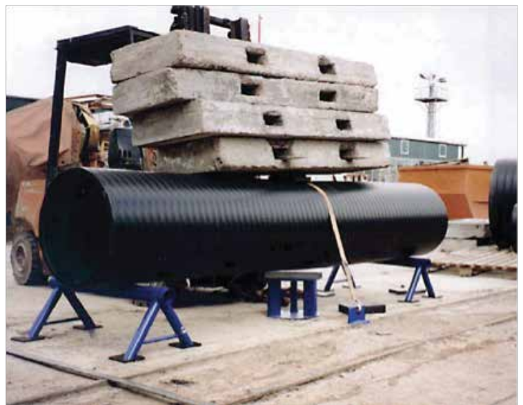
Lengthwise stiffness test for a DN/ID 600mm, SN4 pipe. Load 29kN, deflection 30mm, pipe deformation 54mm.
