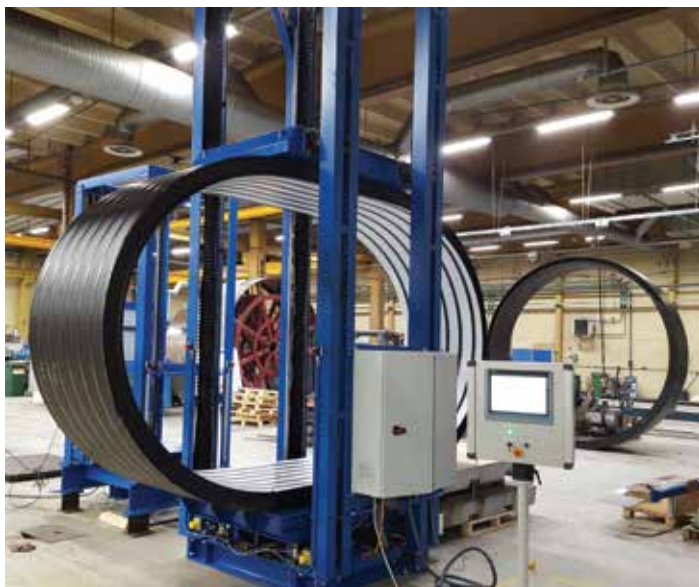
Ring Stiffness Testing of Plasco Weholite Pipes according to ISO 9969 Standard
